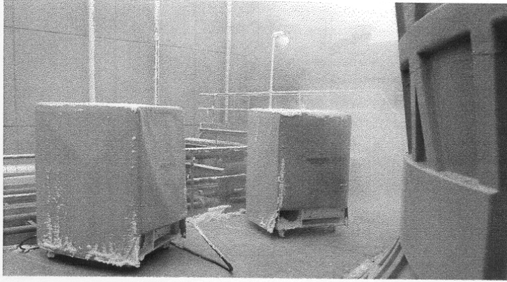
FIGURE 4: Active System Transducers. Loudspeakers designed to withstand hostile environment.
